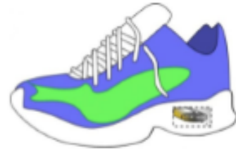
Figure 3: A variation where the piezoelectric element is inside the sole instead of directly above it. This leads to less mechanical stress in contrast.
